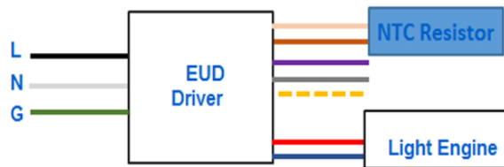
Figure 34: Adding NTC Thermistor for External OTP
